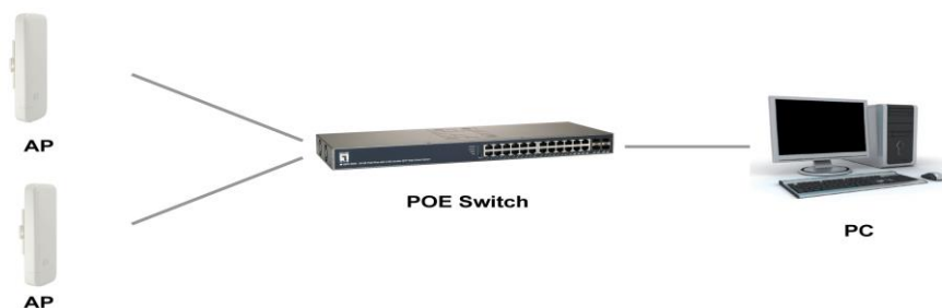
P2 Connection diagram of CPE and PoE
