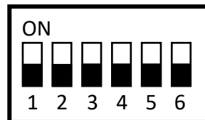
Bild 34 DIP Switch Charge Controller Home & Semipublic
