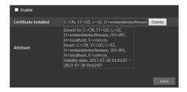
There is a certificate installed by default as shown above. Enable this function and save it. Then the camera can be accessed by entering <a href="https://IP address:https">https://IP address:https</a> port via the web browser (eg. <a href="https://192.168.1.150:443">https://192.168.1.150:443</a>).
