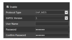
To use this function, the camera shall be connected to a switch supporting 802.1x protocol. The switch can be reckoned as an authentication system to identify the device in a local network. If the camera connected to the network interface of the switch has passed the authentication of the switch, it can be accessed via the local network.
