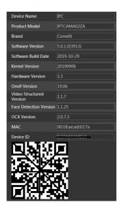
Some versions may support device ID and QR code. If P2P is enabled (see Network Configuration-P2P), the network camera can be quickly added to mobile surveillance client, by scanning the QR code or entering device ID.
