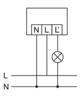
Standard operation with additional connection of external loads
