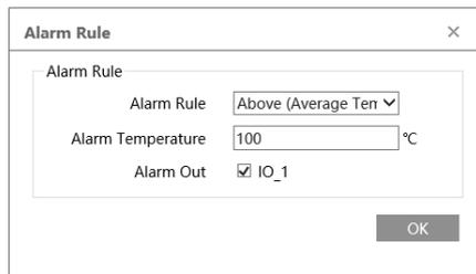
The screenshot shows a dialog box titled "Alarm Rule" with a close button (X) in the top right corner. Inside the dialog, there are three fields: "Alarm Rule" with a dropdown menu set to "Above (Average Tem)", "Alarm Temperature" with a text input field set to "100" and a degree Celsius symbol, and "Alarm Out" with a checked checkbox and the label "IO\_1". An "OK" button is located at the bottom right of the dialog.
