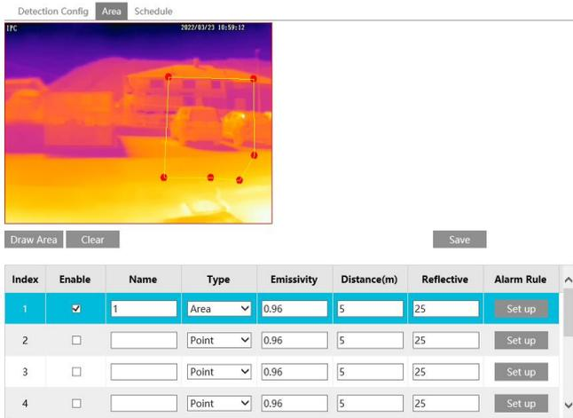
The screenshot shows a software interface for configuring detection settings. At the top, there are tabs for "Detection Config", "Area", and "Schedule". Below the tabs is a thermal image of a building with a red-outlined area drawn on it. Below the image are buttons for "Draw Area", "Clear", and "Save". Below the image is a table with the following columns: Index, Enable, Name, Type, Emissivity, Distance(m), Reflective, and Alarm Rule.
