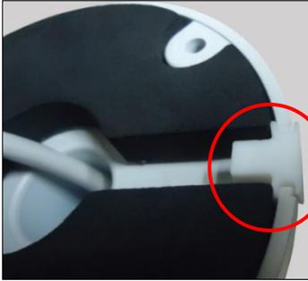
Please mount the rubber plug into the gap of the mounting base
