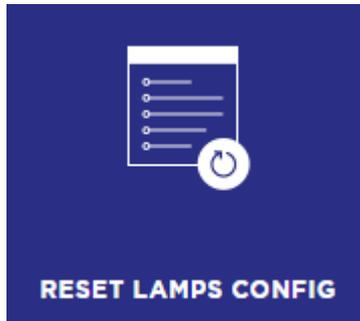
Go to the "OPTIONS" tab and press the "RESET LAMPS CONFIG" button. With this we ensure that the Gateway does not have any previous configuration.
