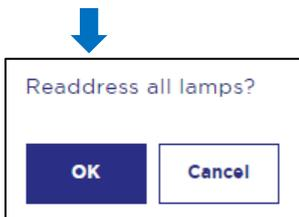
Confirm that you want to assign a new DALI address to all ECGs connected to the Bus.
