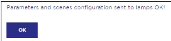
Both the Group configuration and the ECG Parameters and Scenes, or Groups, enabled and configured in the ETS previously are sent to the lamps. If no configuration has been previously uploaded from the ETS, the luminaires will not receive this information.
