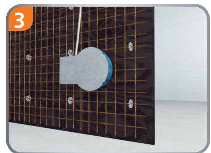
3 Insert the concrete pipes and you can pour the concrete.
