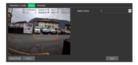
Set the alarm area number on the right side. Up to 4 alarm areas can be added. Click the "Draw Area" button and then click around the area where you want to set as the alarm area in the image on the left side (the alarm area should be a closed area). Click the "Stop Draw" button to stop drawing. Click the "Clear" button to delete the alarm area. Click the "Save" button to save the settings.
