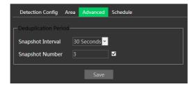
Snapshot Interval: if eg. 5 seconds is selected, the camera will capture the same target once every 5 seconds during its continuous tracking period.
