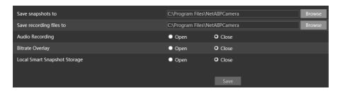
Additionally, the snapshots triggered by smart events (including face detection, line crossing detection and intrusion detection) can be selected to save to the local PC.
