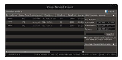
③ Modify the IP address. The default IP address of the camera is 192.168.1.150. Click the information of the camera listed in the above table to show the network information on the right hand. Modify the IP address and gateway of the camera and make sure that its network address is in the same local network segment as the computer's.
