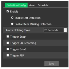
1. Enable object removal detection and then select the detection type.
