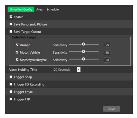
1. Enable region entrance detection and select the snapshot type and the detection target.
