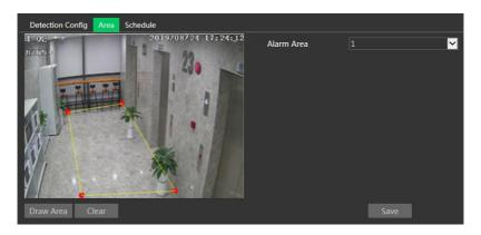
Set the alarm area number on the right side. Up to 4 alarm areas can be added. Click the "Draw Area" button and then click around the area where you want to set as the alarm area in the image on the left side (the alarm area should be a closed area). Click the "Stop Draw" button to stop drawing. Click the "Clear" button to delete the alarm area. Click the "Save" button to save the settings.
