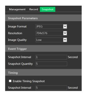
Set the format, resolution and quality of the image saved on the micro-SD card, the snapshot interval and quantity and the timing snapshot here.
