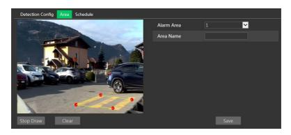
Set the alarm area number and then enter the desired alarm area name. Up to 4 alarm areas can be added. Click "Draw Area" and then select the area where you want to set as the alarm area in the image (the alarm area should be a closed area). Click "Stop Draw" to stop drawing. Click "Clear" to delete the alarm area. Click "Save" to save the settings.
