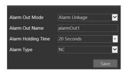
**Alarm Out Mode**: Alarm linkage, Manual Operation, Day/Night Switch Linkage or Timing.
