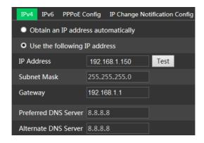
Use IP address (IPv4 for example). There are two options for IP setup: "Obtain an IP address automatically" (by DHCP) and "Use the following IP address".
