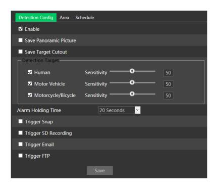
1. Enable intrusion alarm and select the snapshot type and the detection target.
