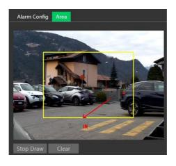
Click "Draw Area" and drag the mouse to draw a rectangle area. Drag the four border lines or the four corners of the rectangle to modify its size. Click "Stop Draw" to stop drawing the area. Click "Clear" to clear the area. Click and drag the arrow or the other end of the arrow line to change the people entrance direction. The size range of the image (width or height) shall occupy from 1/5 to 1/2 of the drawn detection area. The direction of the red arrow is entrance.
