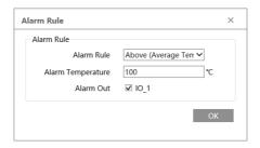
Set the alarm rule, alarm temperature and alarm output. For example, select Alarm Rule as Above (Average Temperature), set the alarm temperature to 100°C and check alarm output.
