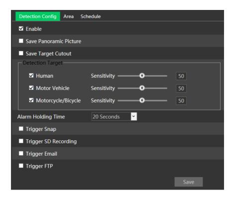
1. Enable region exiting detection and select the snapshot type and the detection target.
