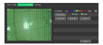
Move the "Sensitivity" scroll bar to set the sensitivity. Higher sensitivity value means that motion alarm will be triggered more easily.
