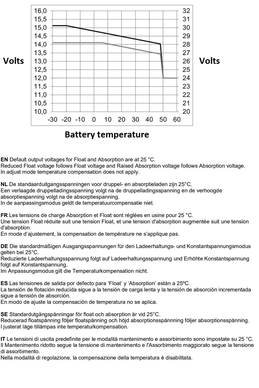
**EN** Default output voltages for Float and Absorption are at 25 °C.
