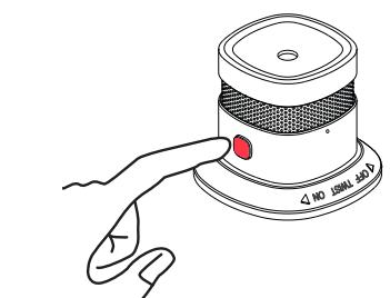
To test or to mute the alarm, press and hold the Test / Mute button for 3 seconds.
