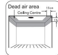
The preferred location to install the smoke detector is in the centre of the ceiling because smoke, heat and combustible products rise to the ceiling and will laterally spread. Keep at least 30 cm distance from lights and decorations and at least 15 cm distance from walls and corners.
