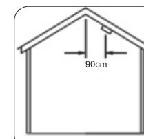
Please install the smoke detector at 90 cm horizontal distance from the ceiling top.
