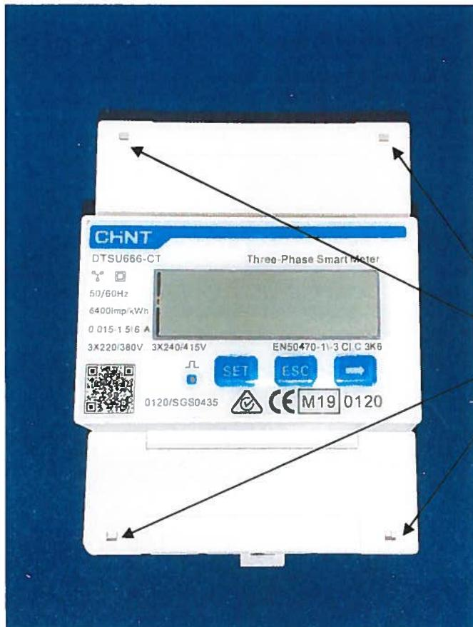
**Terminal cover sealing points**
